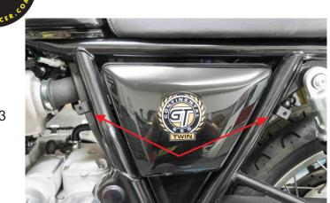
Place the part /accessory as shown in the left hand photo. You will have to twist it parallel to the tube so that it will clip in place.
