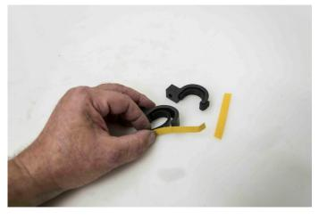
Stick the foam tapes (2x10x80) on all four clips as shown in the photo on the left
