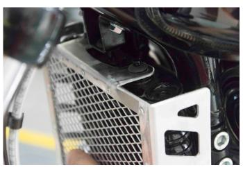
Place the rubbers that you will find in the installation package as shown in photo 3 and in the same way place the new radiator grill in its position.
