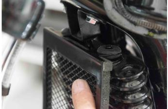
Undo the screws as shown in photo 1 and pull upwards and out your current radiator grill.
