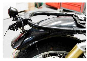
Join the flash light fuses and place them carefully under the small cover, being careful not to mangle them with the cover. If you already have a flash light, the wire will have to slide through the right hand side of the cover and through the notches of the plastic cover — the same as the flash lights
