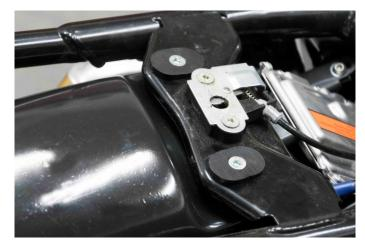
Put the oval plugs in the equivalent notches before sliding through the fender and slightly tightening the nuts that hold the fender in place. Do not forget to place the wire in its previous position.
