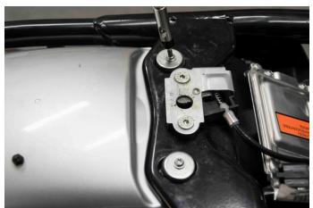
Remove the seat cover and unclip the fuse that powers up the tail lights (photo 1). Then undo the screws that hold the front fender in place (photo 2).
