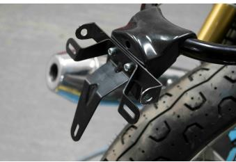
.Put the plastic cover in position as you see in the photo , and do not forget to use the screw (RED arrow in the photo -M6X20 hexagonal washer) as you will not be able to do so later.
