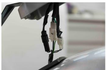
Proceed by removing the screws as shown with the arrows in photo No3. The fender will be released and all you have to do is to unclip the fuse of the tail lights
