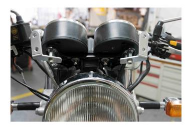
Put the metallic plates in position as shown in the left hand photo.
