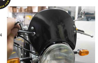
Finally place the mask in position and gradually tighten the screws one by one along with the equivalent nuts.
