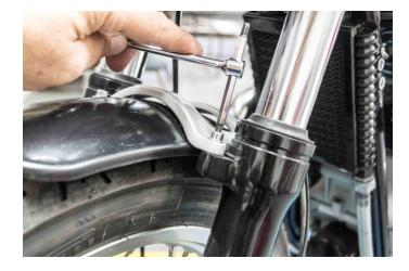
Make sure you tighten the new fender in place.
