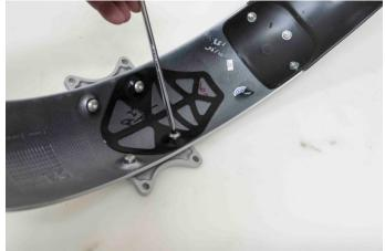
Turn the fender upside down and remove the bridge from the plastic cover.
