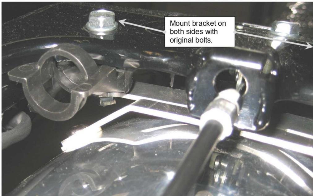
Align fender to the middle and tighten all bolts at last.
